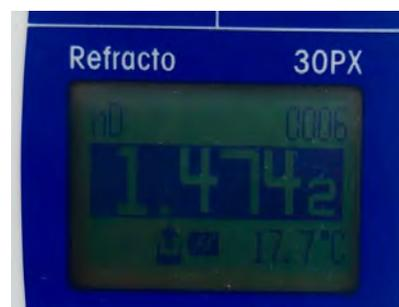
**Figura B16***Resultado P1 – Prensado en Frío*
