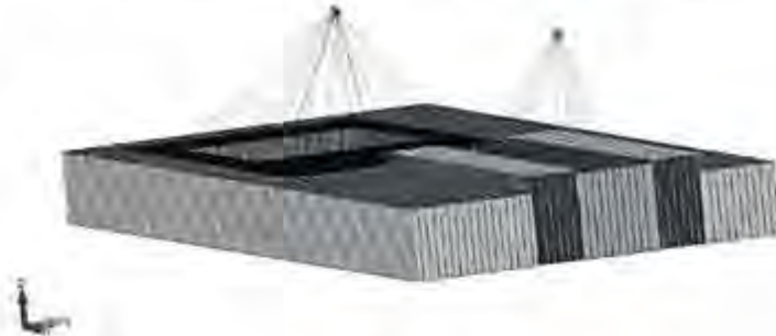
Fig. 6.3.3.3—Finite element model of inertia block and machine (image courtesy of GERB Vibration Control Systems, Inc.).
