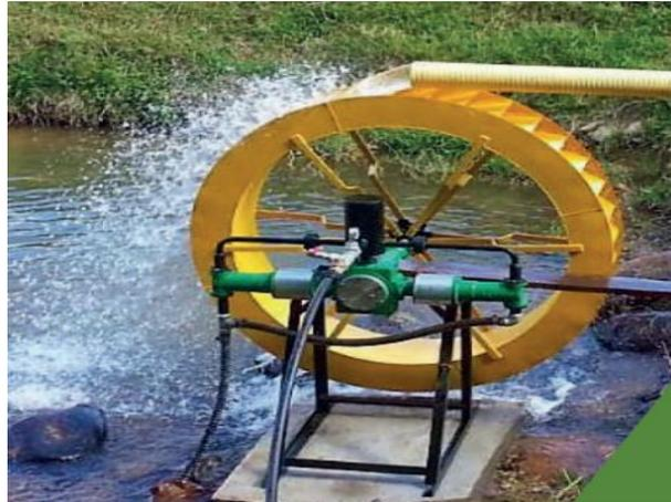
*Nota.* En la figura 7 se observa otro tipo de bomba hidráulica. Tomado de la página web Croper, [https://croper.com/products/10260-bomba-de-pistones?srsId=AfmBOoo4iNI15ZtII1Lc0ByxsM-bKu4L3QgvbpWQB6CwWxNfQx9\\_2zy](https://croper.com/products/10260-bomba-de-pistones?srsId=AfmBOoo4iNI15ZtII1Lc0ByxsM-bKu4L3QgvbpWQB6CwWxNfQx9_2zy)
